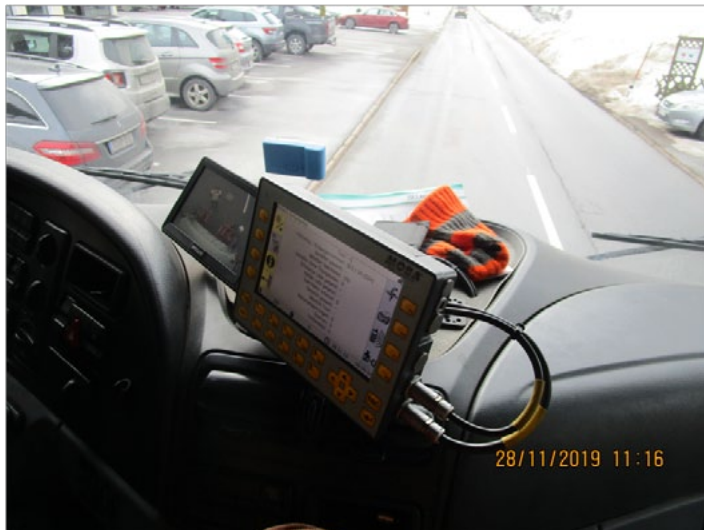
Fig. 3a: Screen from the van cabin, where it is possible to check how many time a dumpster has been emptied and how much do they weight. Photo by Riccardo Maniscalco
